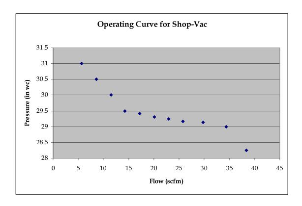
Note to teams: The shop vac was testing with a considerable leak at the exit flange. It is preferable to run the Gas Source without plugging the leak, however, if your design requires additional pressure, we will be prepared to 'plug the leak' for the duration of a short test. Rest assured that we are prepared to help you in all ways possible to help fluidize your prototype
